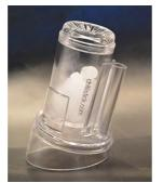
The filled ice cage is pushed into the **pour top** with the valve of the **Ice Cage** facing downwards. Please note that at room temperature the grip feature in the **Pour Top** appears too firm to accommodate the **ice cage** however once chilled by the dry ice it will fit well.
