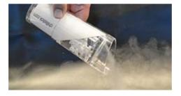
When tilted as described the essence will mix with the dry ice at which point the liquid will be atomized and will flow out of the device. The cloud created will be perfumed with the chosen essence.
